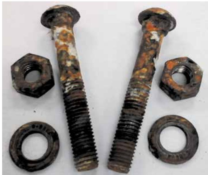
Figure 5: Zinc-electroplated carbon steel hardware after 1000hr C5-M salt spray testing
